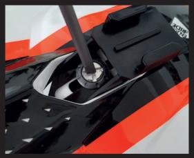
Once the GoPro® mount is in the correct position, tighten the screw with a screwdriver.
