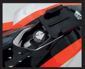
Use the mount in as close as possible to the position shown in the photo. In this way it will be guided by the visor and won't rotate while using the camera on top of the mount.
