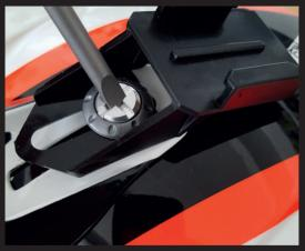
Use a screwdriver to turn the screw into the thread of the helmet.
